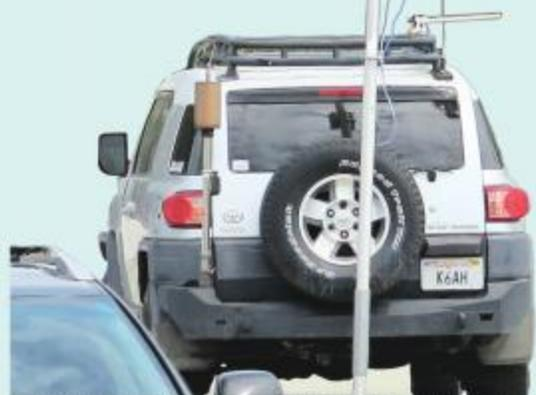
*K6AH mobile nodes with dish and sector antennas*
