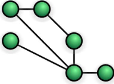
Illustration of a **partial mesh** network. A fully mesh network is where each node is connected to every other node in the network.
